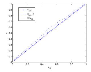
Fig. 4. Experimental evaluation: comparing lower bound on degraded speed (dotted line) with average computed value (solid line) and average plus standard deviation (dashed line).
