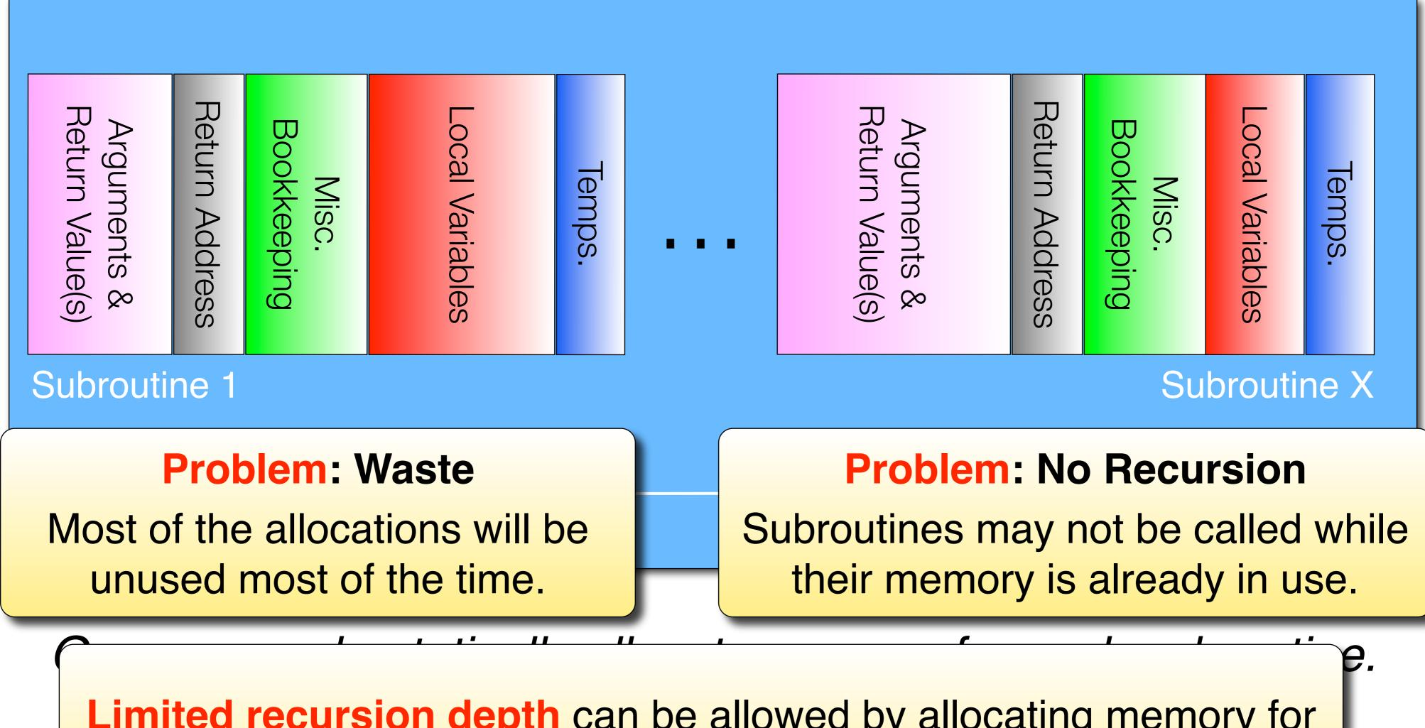
Limited recursion depth can be allowed by allocating memory for multiple subroutine *instances*. But this increases waste...
