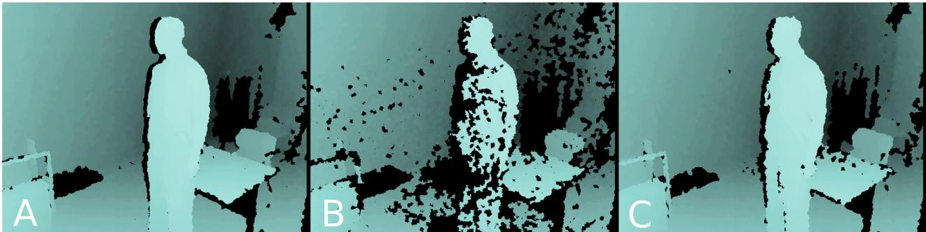
Figure 1: Left to Right: A) Depth map of room using a single Kinect. B) Depth map with 5 additional Kinects overlapping the view, causing prominent interference holes. C) Depth map with 5 additional overlapping Kinects while applying our interference reduction technique.
