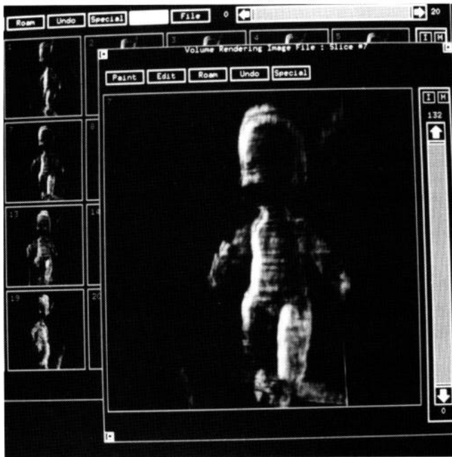
Figure 2. Reconstructed and rendered image of the toy doll phantom using incremental volume visualization.
