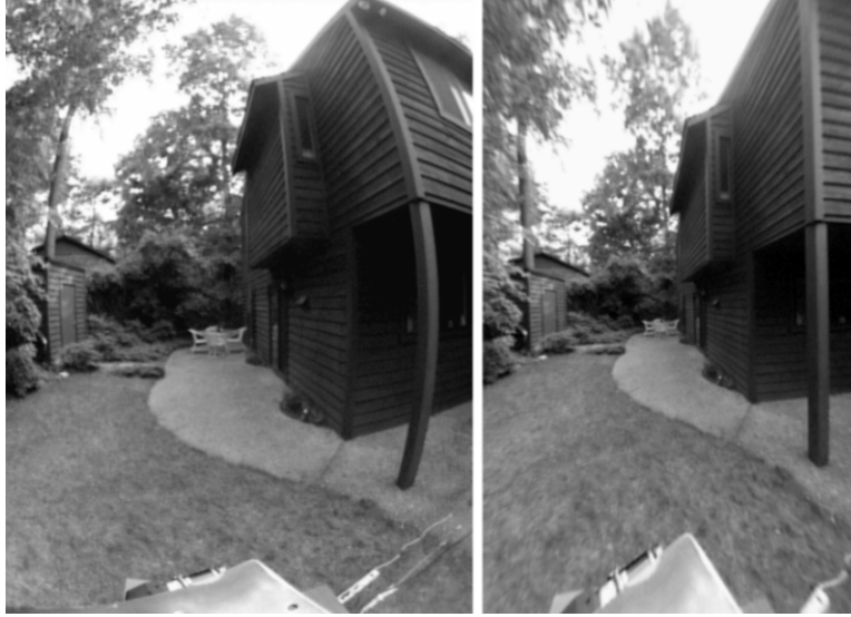
Figure 4-14: A fisheye (left) and planar (right) projection of a yard scene
