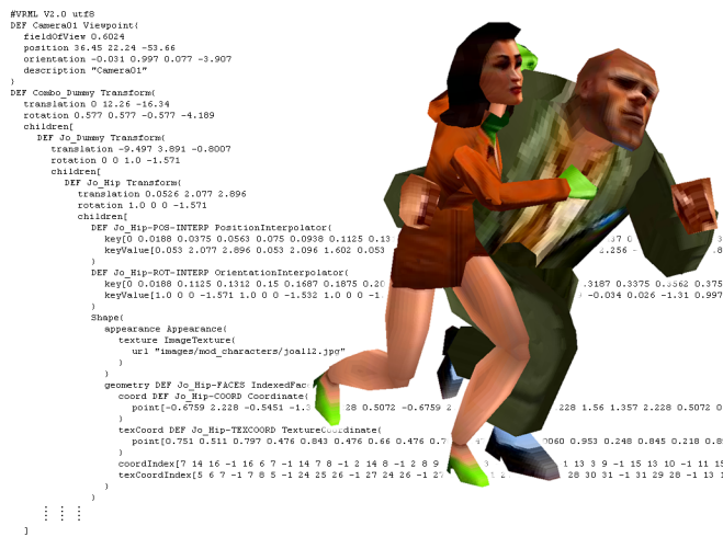
Figure 1. Our example VRML scene contains 33 indexed face sets, 5 position interpolators, and 27 orientation interpolators. The size of the gzipped VRML file is 29895 bytes. With ASCII coded indexed face sets this reduces to 18364 bytes. Additional ASCII coding of all interpolators brings it down to 12996 bytes.
