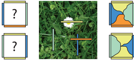
Figure 24: Left : Two tiles with four different border constraints must be created. Middle : A position for each colored edge is chosen in the source image. This defines the content that will appear along each edge. Right : Each edge provides a positioning of the source image in the tile. Graph cut optimization is used to find optimal transitions between the edges. (Several variants are possible, such as adding a patch in the center of the tile to increase visual variety).
