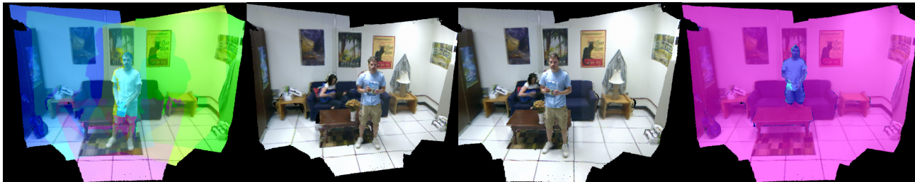
Figure 1. Left: Color coded contribution of the five Kinect sensors used in test system. Two center images: Two views of a live capture session. All surfaces displayed are captured dynamically. Right: Raytracing of 3D Volume Segmentation. Pink indicates background, blue indicates foreground, cyan indicates scene motion, and black represents unknown (no data).
