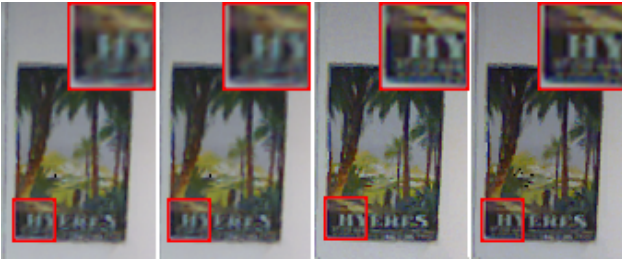
Figure 5. Texture quality. Left to right: 1) voxel coloring at 384 \times 268 \times 268 and 2) 875 \times 612 \times 612 volume resolution, 3) projective texture mapping at 384 \times 268 \times 268 and 4) 875 \times 612 \times 612 volume resolution.
