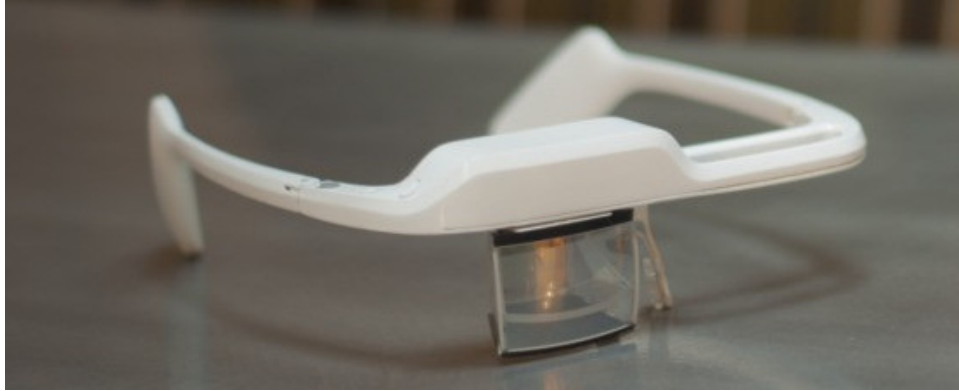
Figure 2.4: Example of combined reflective design head-mounted display, the Laster SeeThru. Photo by Laster.
