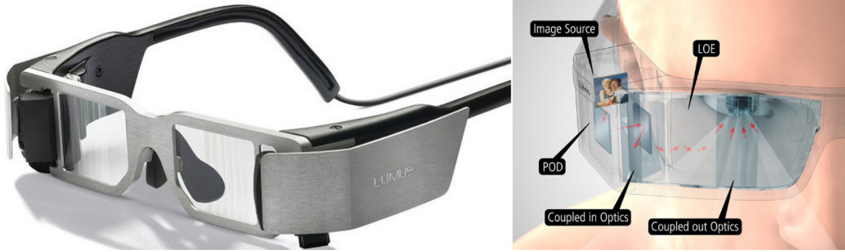
Figure 2.6: Left: Example of waveguide design head-mounted display, the Lumus DK-32. Right: Diagram showing Lumus optical components including the LOE (Light-guide Optical Element), i.e. a waveguide, and the POD, which projects the image source into the waveguide. Photo and diagram by Lumus.
