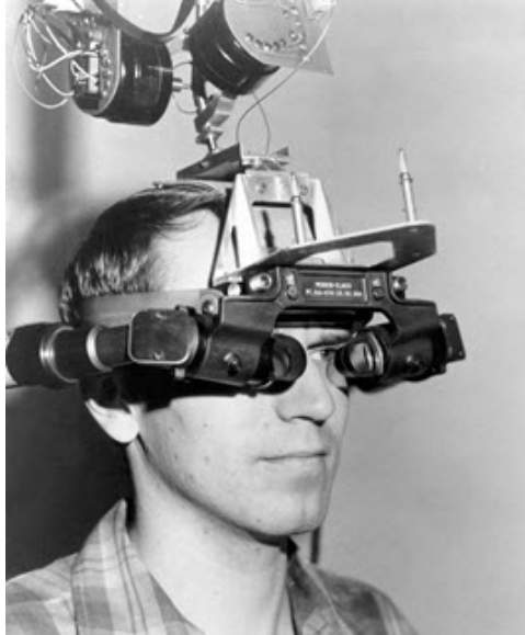
Figure 2.3: Example of simple combiner head-mounted display used in a system by Sutherland (1968).
