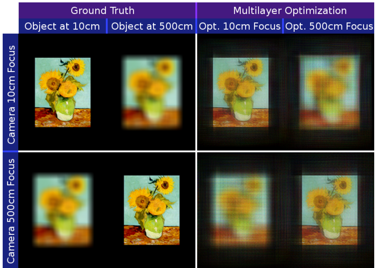
Figure 3.7: Multiple focal position simulation. Synthetic objects at different focal depths can be displayed simultaneously on the display. Top row: Light field refocused with synthetic camera at close (10 cm) focus. Bottom row: Light field refocused with synthetic camera at far (500 cm) focus. Left column: Original light field, provided as input to the optimization process. Right column: Simulated reconstructed views using multilayer optimization. Optimization was performed with two layers, eight time-multiplexed frames, brightness scaling factor \beta = 0.1 (see Section 3.5.4) and the geometry of the prototype display (see Section 3.6).
