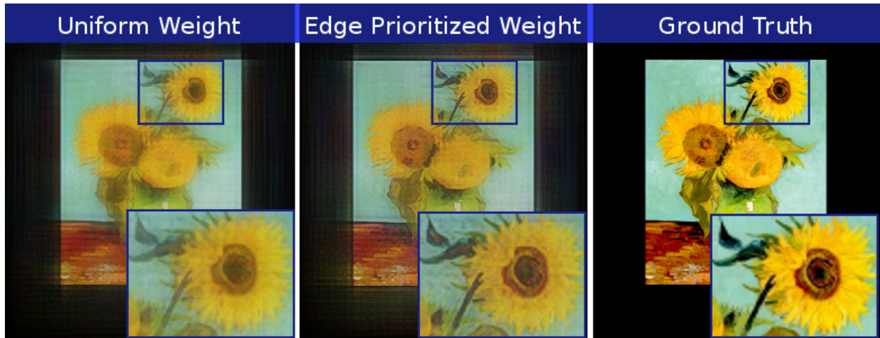
Figure 3.10: Perceptual Optimization. Left : Simulated light field reconstruction using uniform ray weighting. Center : Simulated reconstruction using ray weighting based on contrast with adjacent rays. Right : Original light field, used as input to the optimization process. Inset images show magnified region of topmost flower. Note improved contrast of green stem and leaves when using edge prioritized weights (center) as compared to use of uniform weights (left). Optimization was performed with two layers, eight time-multiplexed frames, brightness scaling factor \beta = 0.1 (see Section 3.5.4), a focal distance of 15 cm and the geometry of the prototype display (see Section 3.6).
