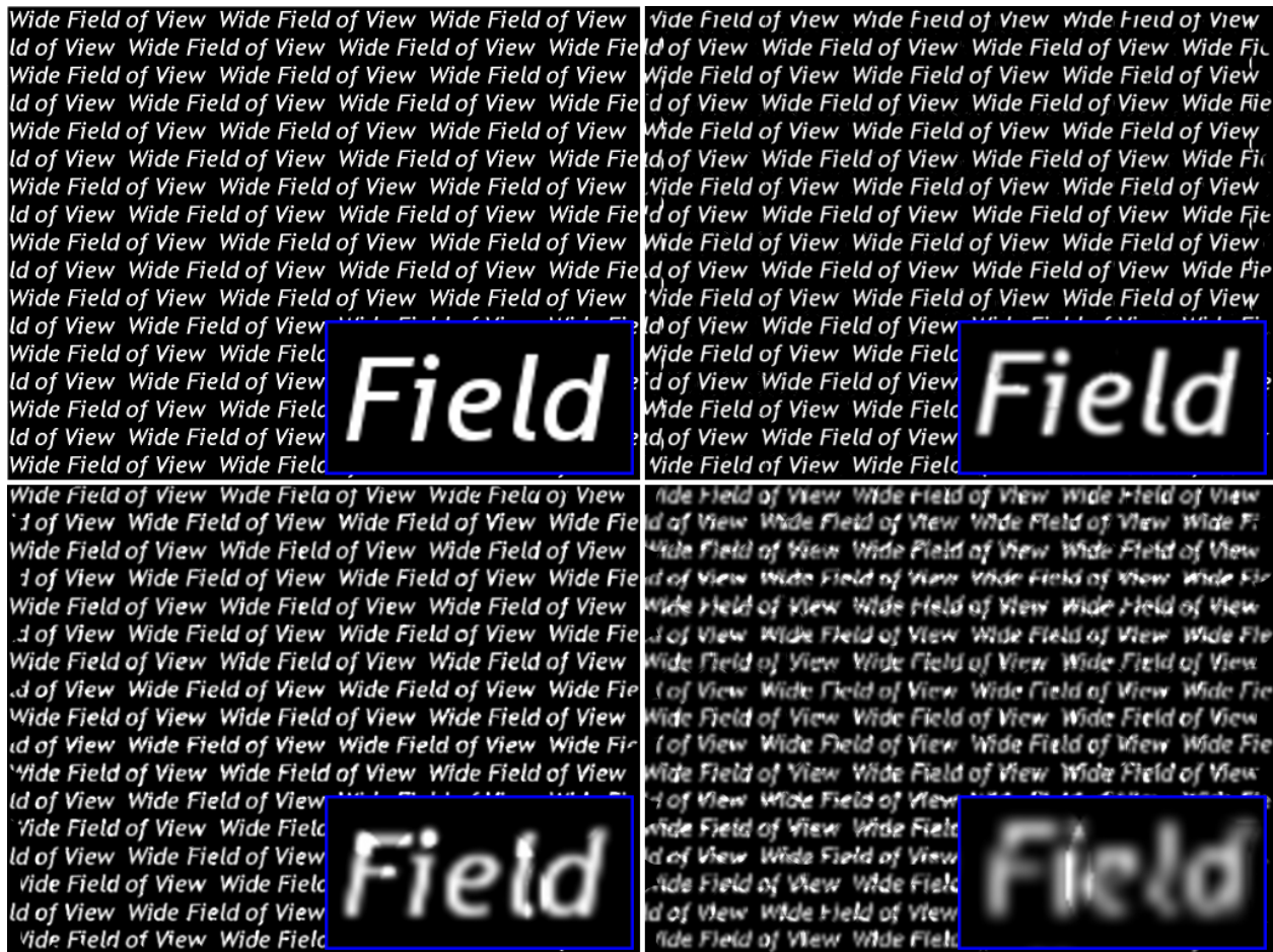
Figure 4.19: Display simulations. Outlined inset images show magnified regions. Top Left: Reference image, used as target image for simulation. Top Right: Tracked configuration simulation. Bottom Left: Untracked configuration simulation (small eyebox). Bottom Right: Untracked configuration (larger eyebox).
