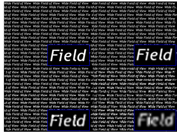
Figure 9: Display simulations. Blue outlined inset images show magnified regions. Top Left: Reference image, used as target image for simulation. Top Right: Tracked configuration simulation. Bottom Left: Untracked configuration simulation (small eyebox). Bottom Right: Untracked configuration (larger eyebox).
