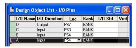
Save the pin assignments entered into the PACE tool, and exit that window. The PACE tool just manipulates a text file, so another way to enter pin assignments is to edit the text file directly using the *Edit Constraints (text)* command. *Optional:* If you double-click on Edit Constrains, you'll see a file with these contents.
