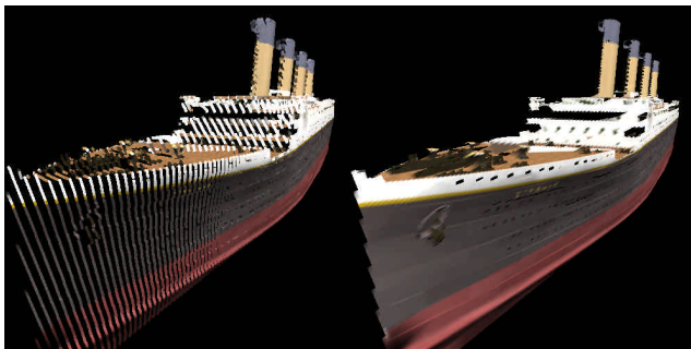
Figure 15 The image on the left is constructed by splatting every fourth column in the MCOP dataset. This shows the image-slices acquired by each camera on the curve. On the right is the dataset rendered by connecting adjacent points with triangles.
