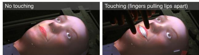
Figure 1: Our touch-sensitive physical-virtual head for hands-on healthcare training. The prototype comprises a translucent head-shaped shell with a digital projector, IR light sources, and cameras underneath. Left: No touch. Right: A nurse diagnosing a potential stroke uses her fingers to pull the lips apart to inspect the gums.
