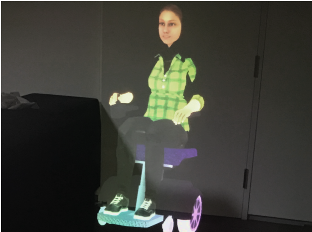
Figure 1: Photo taken through a Microsoft HoloLens optical see-through head-mounted display showing a virtual human (in a wheelchair) entering the room by driving through a closed physical door in a “ghost-like” fashion, i.e., the virtual human’s more distant body parts are occluded by the door.
