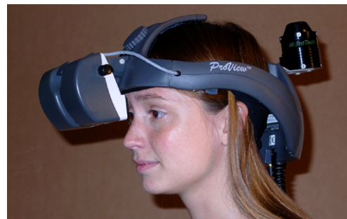
Figure 3. A user wearing a Kaiser ProView™ 30 HMD. Her peripheral vision is unobstructed.
