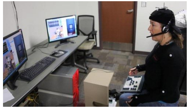
Figure 4: Puppetry controlled by upper body and head motion capture. Foot buttons are used for facial expressions and Ergodex for agent behaviors. Interactor's monitors have two windows: one shows virtual content as seen by user; the other window displays a video of the user.
