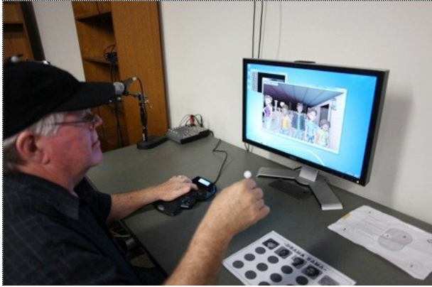
Figure 6: Puppetry controlled by a pawn (single retro-reflective marker on a post), head tracking and a game pad. Note the template on the desk. This was used in studies that employed puppetry for experiences that dealt with peer pressure and cross cultural interaction.
