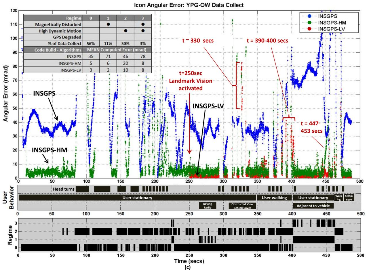
Figure 11. Data collect YPG-OW using the testbed system: (a) snapshots capturing user behavior during sequence, (b) representative helmet kit camera images for user adjacent to vehicle with ground truth coordinate (red dot) and rendered icon position for INSGPS-HM-LV algorithms, and (c) icon angular error plot and reported mean errors for dynamic and magnetic disturbance regimes.
