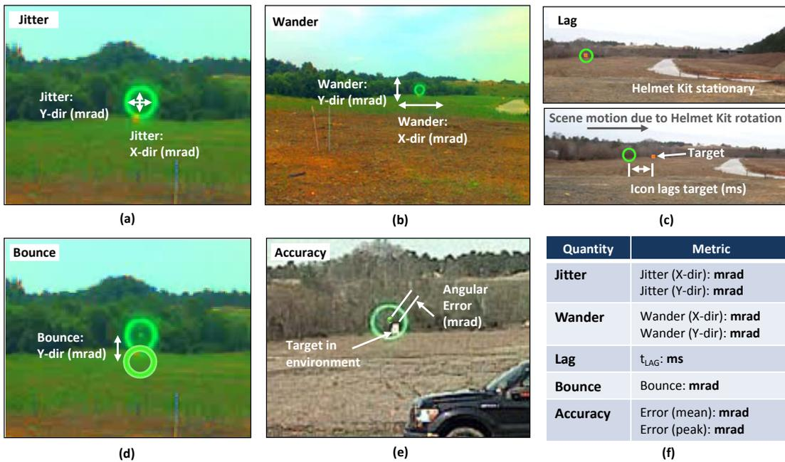
Figure 5. We evaluate algorithm performance against five primary test metrics. We test for (a) jitter, (b) wander, (c) lag, and (d) bounce under specific controlled motion sequences imparted by an automated motion system. We assess (e) accuracy performance over the entirety of body-worn data collects, with the user carrying out motions and behaviors representative of dismounted soldier operations. (f) We report metric results as shown.
