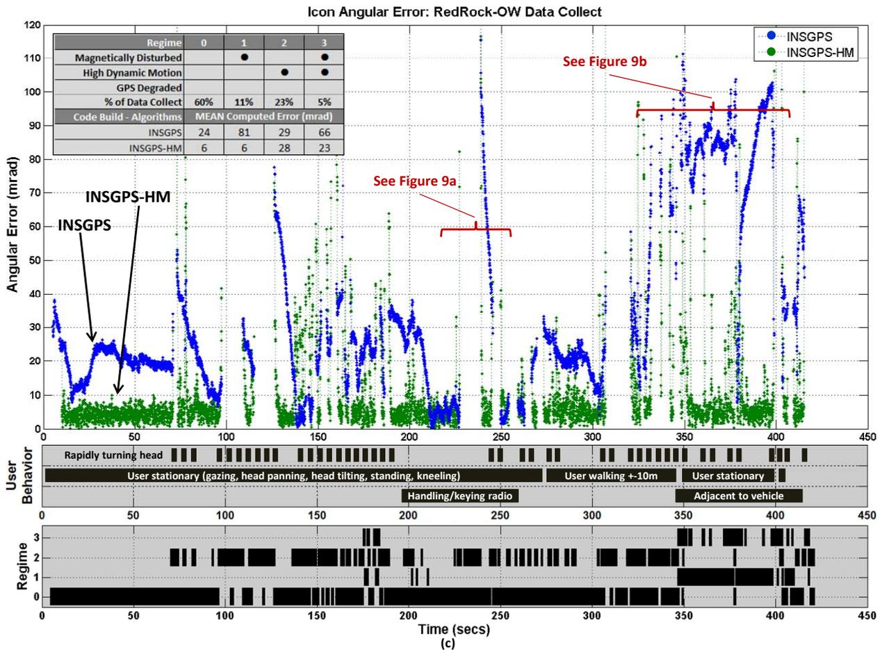
Figure 8. Data collect RedRock-OW using the testbed system: (a) snapshots capturing user behavior during sequence, (b) representative helmet kit camera image with ground truth coordinate (red dot) and rendered icon positions for INSGPS and INSGPS-HM algorithms, and (c) icon angular error plot and reported mean errors for dynamic and magnetic disturbance regimes.
