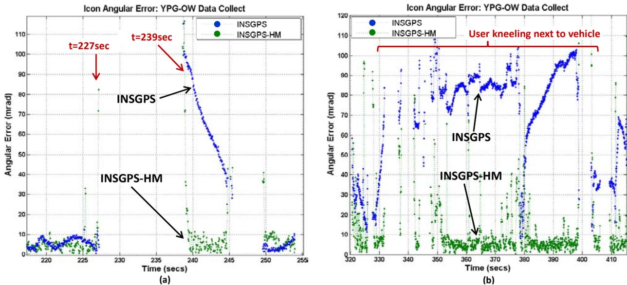
Figure 9. Close-up icon angular behavior for: (a) a head turn/body rotation away from a view of mountainous terrain and (b) user assessment of his environment when kneeling next to his vehicle. Our horizon matching algorithms provide azimuth inputs to the filter that maintain icon angular error below 10mrad for low user dynamics conditions.
