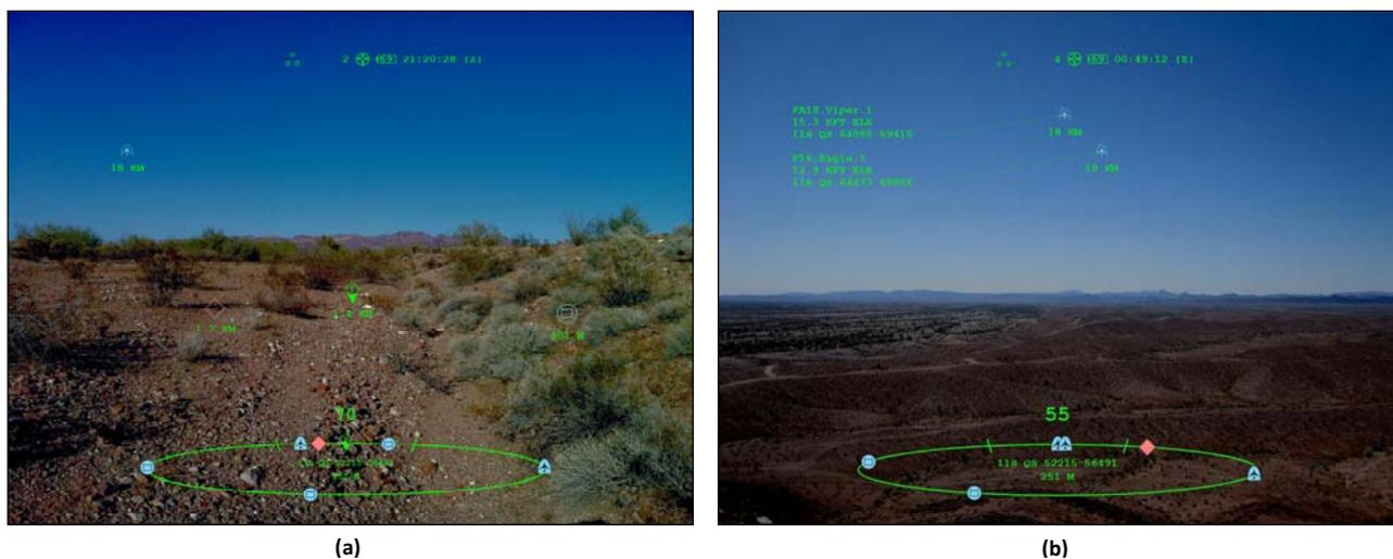
Figure 4. The ULTRA-Vis heads-up user interface offers the potential for enhanced dismount soldier mission effectiveness. (a) A soldier can navigate with increased tempo through real-time understanding of his position, heading, and the locations of waypoints and friendly forces. (b) An operator can more effectively manage and direct aircraft movements via heads-up visualization of icons in his real-world view of the airspace. ULTRA-Vis UI simulation tool shown above.
