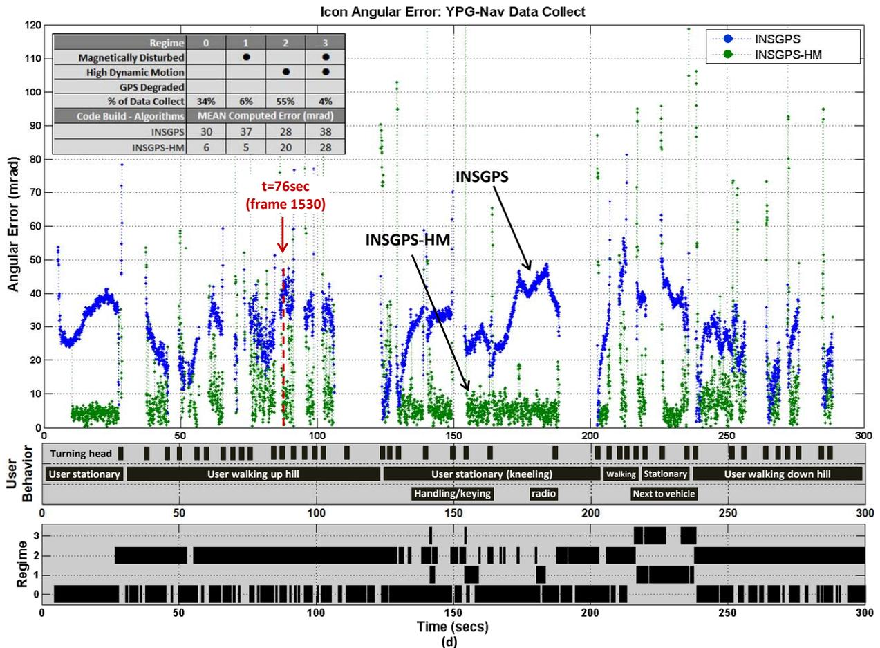
Figure 10. Data collect YPG-Nav using the testbed system: (a) snapshots capturing user behavior during sequence, (b) representative helmet kit camera image with ground truth coordinate (red dot) and rendered icon position for INSGPS-HM algorithms, (c) sequence of consecutive helmet kit camera images (at 20 fps) illustrating degree of icon fluctuation during user walking, and (d) icon angular error plot and reported mean errors for dynamic and magnetic disturbance regimes.
