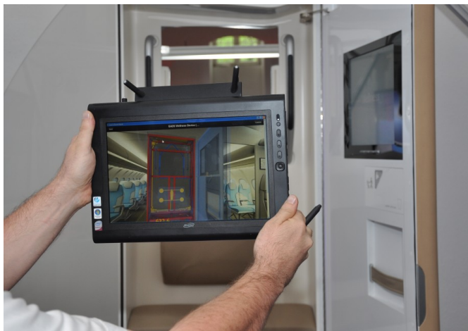
Figure 1.11.: Qualitative discrepancy check. The virtual model of an airplane cabin is rendered from the perspective of the display to allow for a straightforward review of the current state and correctness of the construction process. (Courtesy of EADS Innovation Works [Keit 10b])
