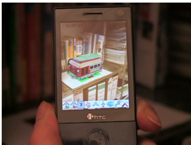
Figure 1.4.: Mobile AR viewer. A virtual object is integrated into the live video of the real scene.
