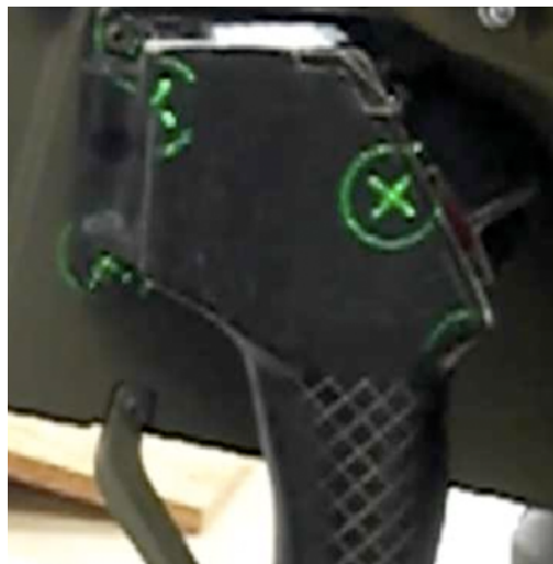
Figure 1.13.: Maintenance instructions projected onto the missile launcher
