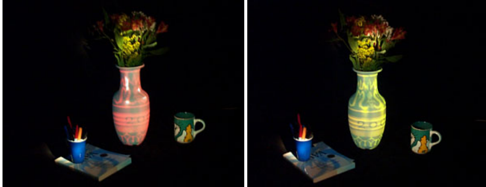
Figure 5.3: The surface appearance of a neutral colored object is changed by 'painting' it with projected light.
