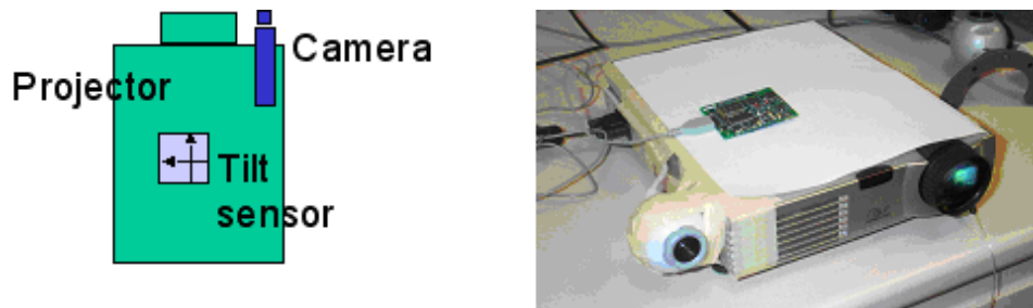
Figure 6.2: Extending the geometric framework to tracked projectors: The projector, augmented with a camera and tilt sensor, can automatically detect relative orientation with respect to a vertical planar screen. The three angles can be used for keystone-correction without the aid of any external devices.
