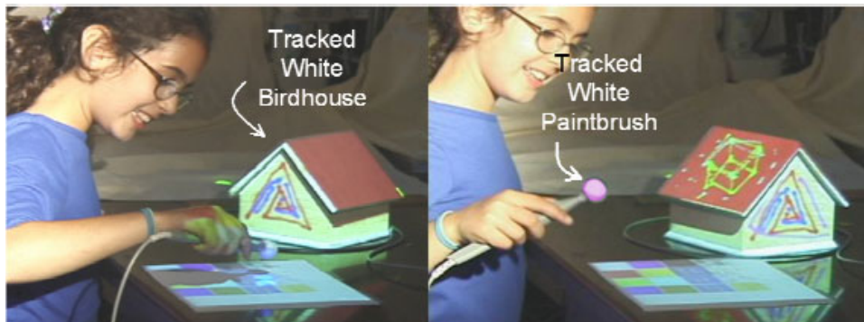
Figure 6.3: Extending the geometric framework to tracked display surfaces: Two projectors illuminate tracked white objects.
