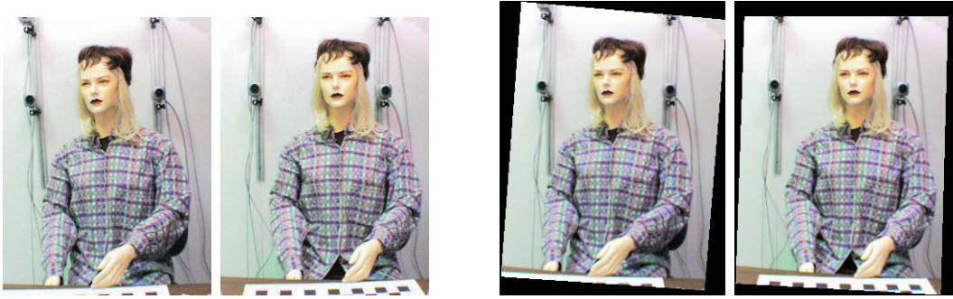
Figure 2.4: A pair of stereo images before and after rectification. The first two are the original images, while the last two are the rectified images. Note that the corresponding features are on the same row of pixels after rectification.
