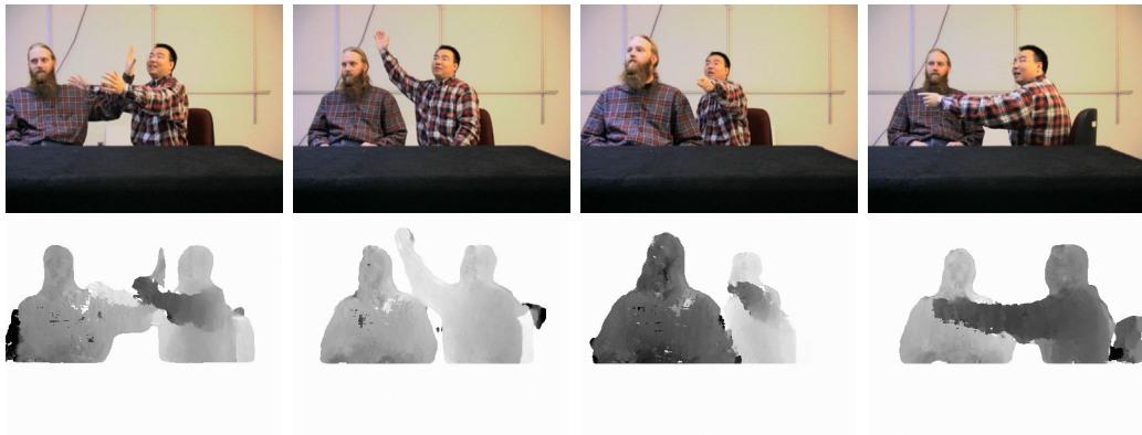
Figure 4.14: More results from our real-time online stereo system. The first row shows the input images; The second row shows the corresponding disparity map.
