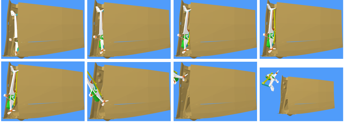
Figure 6.13: Maintainability of the windscreen wiper motion. The first image shows the input configuration for the benchmark, where the wiper is inside the windscreen model with very tight space. The wiper needs to be taken outside with the final configuration shown in the last image. The intermediate sequence of images shows a path automatically computed by D-Plan.
