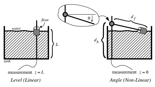
**Figure 5:** The two possible measurement methods. *Left:* the system returns a noisy voltage z representing the *height* of the float. *Right:* system returns a noisy voltage z representing the *angle*  $\theta$  between the fixed base segment  $d_b$  and the pivoting float segment  $d_f$ .
