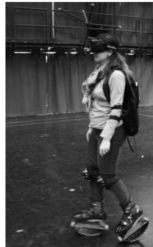
Figure 6: A reproduction of Figure 2 from [28] by Nabiyouni and Bowman at Virginia Tech. © 2015 The Eurographics Association. Reprinted by permission. The figure depicts an experimental subject wearing a tracked head-worn display and a pair of Kangoo Jumps™ boots, which are claimed to provide an effective method for improving aerobic capacity compared to normal running shoes.
