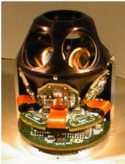
FIGURE 7.9. The HiBall Sensor LEPD Configuration [106]
