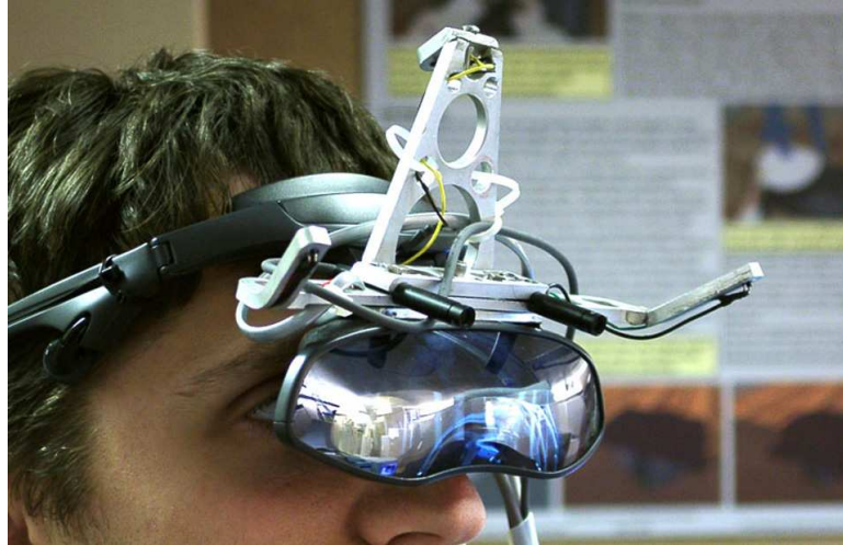
Figure C.3: Video-see-through augmented reality head-mounted display (HMD) built on the basis of a Sony Glasstron LDI-D100 device. The aluminum superstructure holds two miniature video cameras for image capture and three infrared LEDs for opto-electronic tracking of the HMD.
