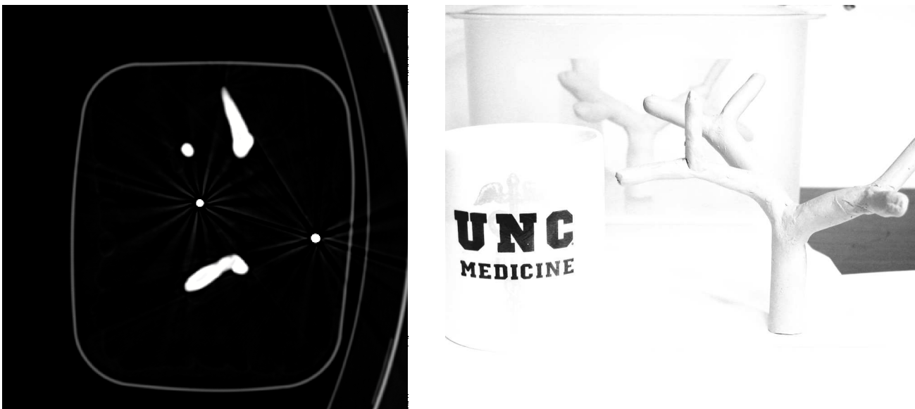
Figure 7.2: CT and optical images of one of the vessel phantoms. The CT image (left) shows segments of the vessel branches as well as slices of the embedded fiducials. The optical image (right) shows the branching structure of the model and its relative size.
