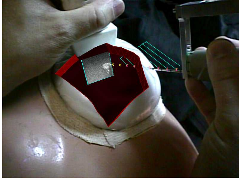
Figure C.2: Head-mounted display view during this phantom biopsy experiment (in 2000). Both the ultrasound probe (left hand) and the biopsy needle (right hand) are tracked. The needle aims at the bright lesion visible in the ultrasound slice. The system displays the projection of the needle onto the plane of the ultrasound slice (blue lines) and also displays the projected trajectory of the needle if it were fired at this moment (yellow markers)
