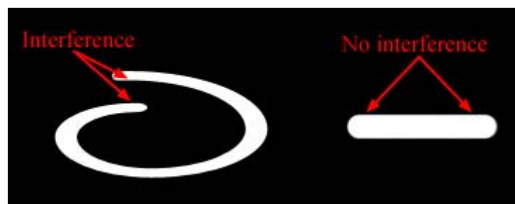
Fig. 7.18. Diagrams showing slices through two different slab-like objects. When dealing with tortuous objects, such as the one on the left, object edges may interfere during core computation if they are close to each other and if the image is noisy. This is not a problem with straighter objects, such as the one on the right.
