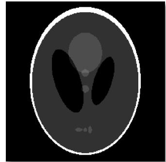
Fig. 146 Matlab’s single-slice “brain” phantom function called with randomly sampled parameters.
