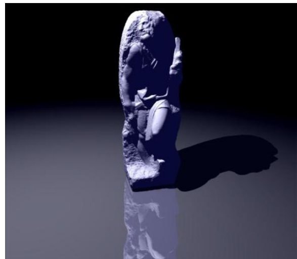
128 million triangle St. Matthew statue rendered at interactive frame rates using our R-LOD approach
