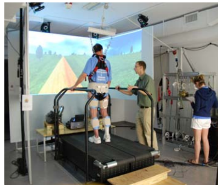
Dual-belt treadmill and three screen VE system in the Human Motion Science laboratory.
