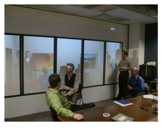
A mockup of a future telepresence wall display using five 65" displays in a typical meeting room.
