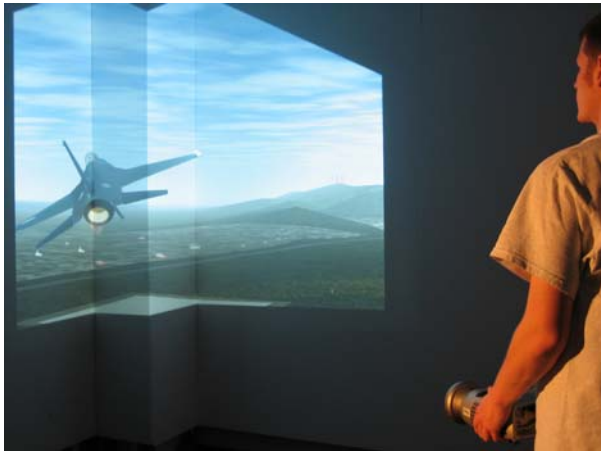
Continuous projector calibration allows the system to compensate for the new location of the projector as it is moved by the user.
