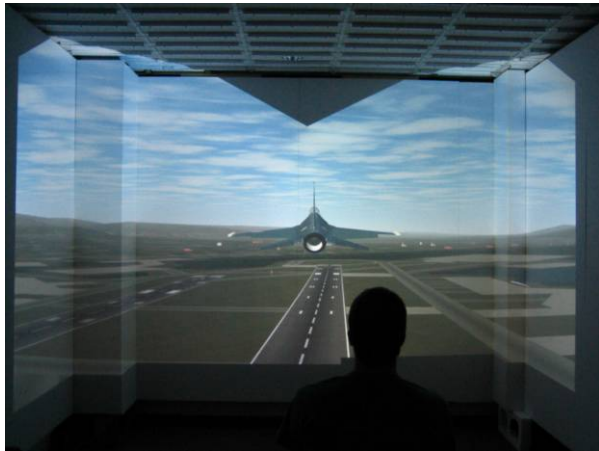
An immersive display in a multi-wall room built with two short-throw projectors.
