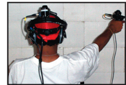
During the game, the virtual hand drifted from the real hand position. Users compensated to maintain a consistent visual scene. This user believes he is aiming at the panels directly in front of him.
