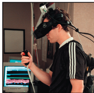
A user wearing a head-mounted display and physiological measuring equipment. Heart-rate is shown in the computer monitor in the lower-left corner.
