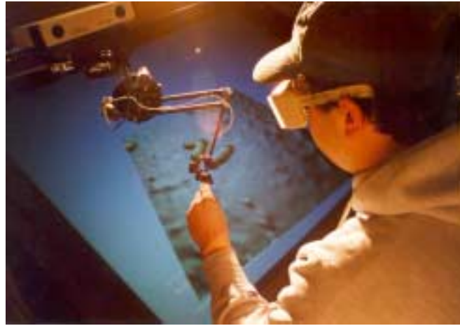
Far left: This model of a man contains 7,152 triangles. It can be "felt" in real time with a PHANTOM using H-Collide with SensAble Technology's GHOST library. Left: a user of the nanoWorkbench examines a particle of tobacco mosaic virus on a representative surface. The surface tested with H-Collide had 12,482 triangles.
