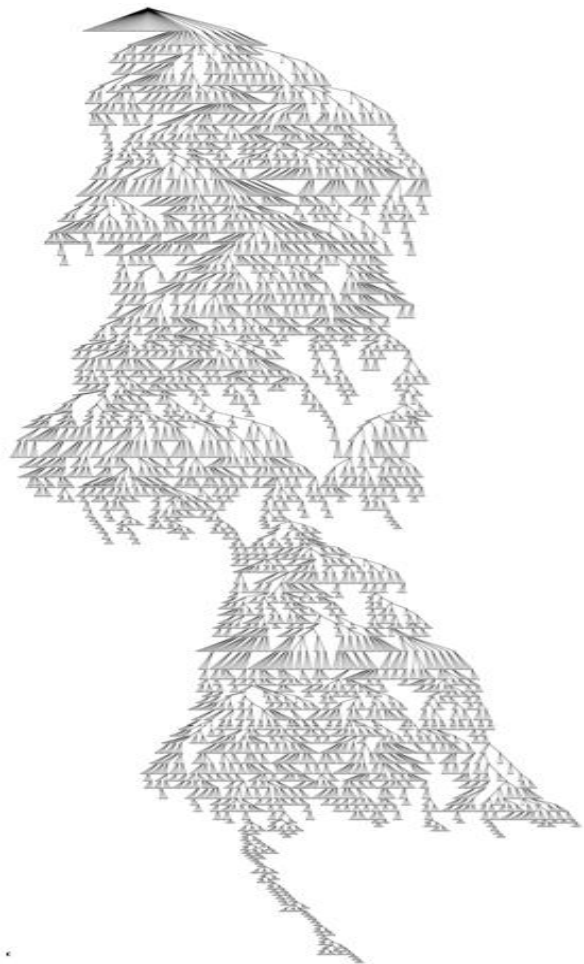
An example of tree-structured computation. Imbalance in the tree necessitates significant load balancing efforts to achieve parallel speedup in a multiprocessor traversal.
