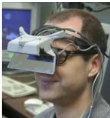
Video see-through HMD built from a modified Sony Glasstron high-resolution stereo unit, equipped with miniature video cameras aligned to the wearer's eyes via mirrors. Left: Parametric design simulation. Right: Finished device (photo by Caroline Green).
