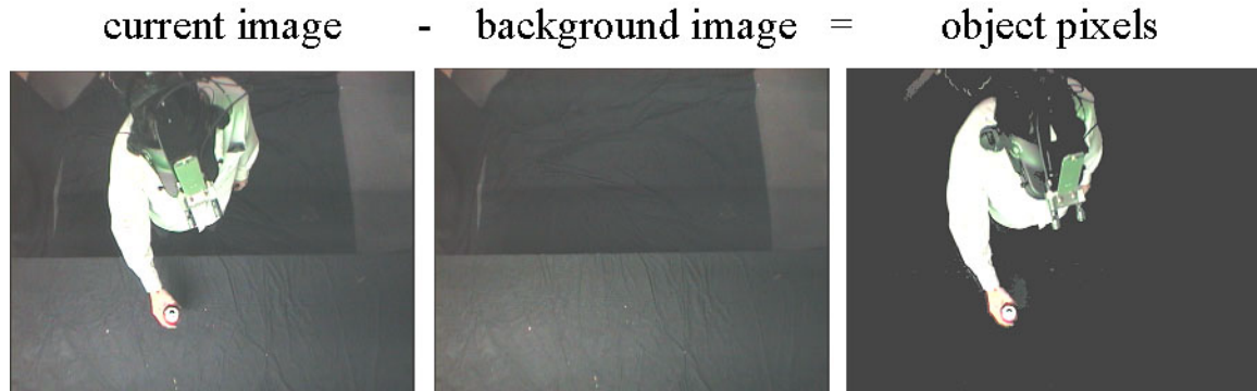
Figure 3 - Frames from the different stages in image segmentation. The difference between the current image (left) and the background image (center) is compared against a threshold to identify object pixels. The object pixel map is stored in the alpha channel. For the right image, we cleared the color component of background pixels to help visualize the object pixels.
