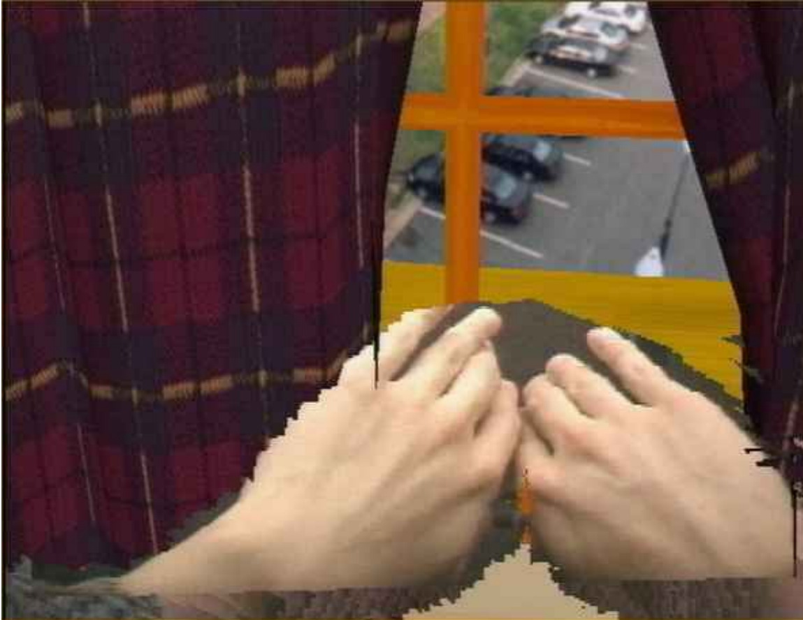
Figure 10 – A participant parts virtual curtains to look out a window in a VE. The results of detecting collisions between the virtual curtain and the real-object avatars of the participant’s hands are used as inputs to the cloth simulation.
