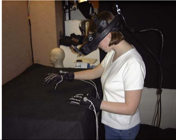
Figure 22 – Purely Virtual Environment (PVE) setup. The user wore tracked pinchgloves and manipulated virtual objects.
