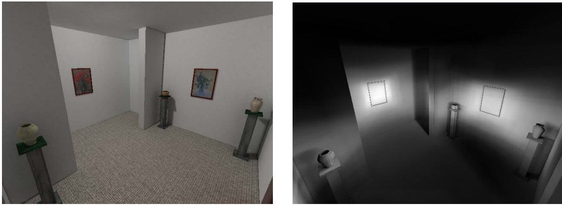
Figure 4.1: VE from user's point of view (left) and the attention-mapped environment (right). Brighter grays indicate longer viewing times.
