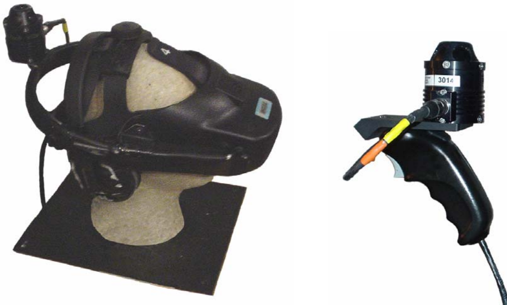
Figure 1.1. Virtual Research V8 HMD (left) and joystick (right). Both pieces of equipment are tracked with a 3rdTech HiBall optical tracking system.
