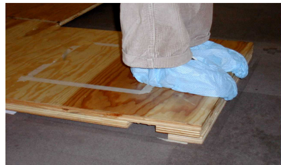
Figure 4. Subject in slippers with toes over 1.5-inch ledge.
