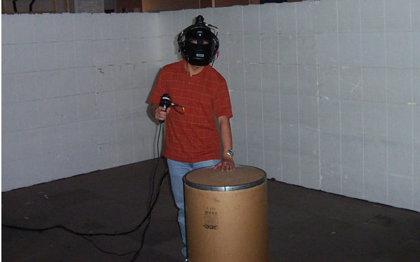
Fig. 2. A user touches the one cylindrical object intended to provide haptic feedback. The Styrofoam walls mark the limits of the tracked space.
