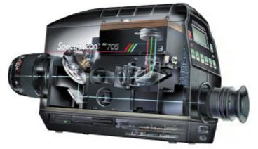
These hardware features make this SpectraScan a self-sufficient, stand-alone instrument. No computer is required to set-up the instrument, make measurements or display the calculated results.
