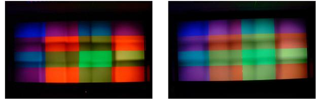
Fig. 1. Left: A display of  $5 \times 3$  array of 15 projectors where the overlap regions are blended by using a physical shadow mask on the light path of the projector. Right: The same display with the overlap region blended by a linear ramp in software. For this, it is necessary to have the knowledge of the exact location of the overlap region. Note that the overlapping regions are distinctly noticeable in both cases.
