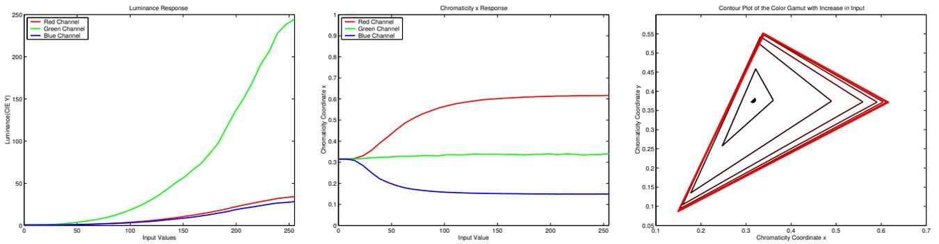
Fig. 2. Left: Luminance response of the three channels. Middle: Chromaticity  $x$  for the three channels. The shape of the curves for chromaticity  $y$  are similar. Right: Gamut contour as the input changes from 0 to 255 at intervals of 32.
