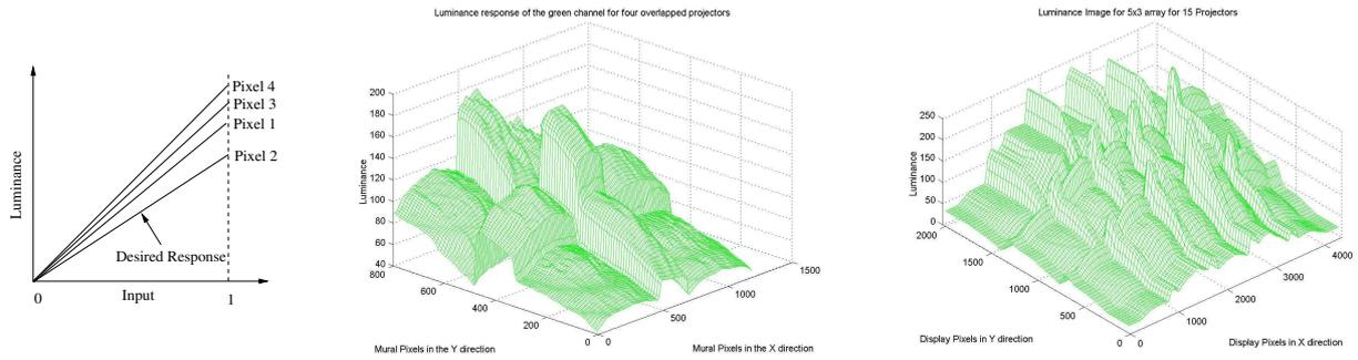
Fig. 12. Left: The common achievable response with four sample pixel response. The response with the least range is the common achievable response. Middle: The display luminance surface for  $2 \times 2$  array of four projectors. Right: The display luminance surface for  $5 \times 3$  array of 15 projectors.
