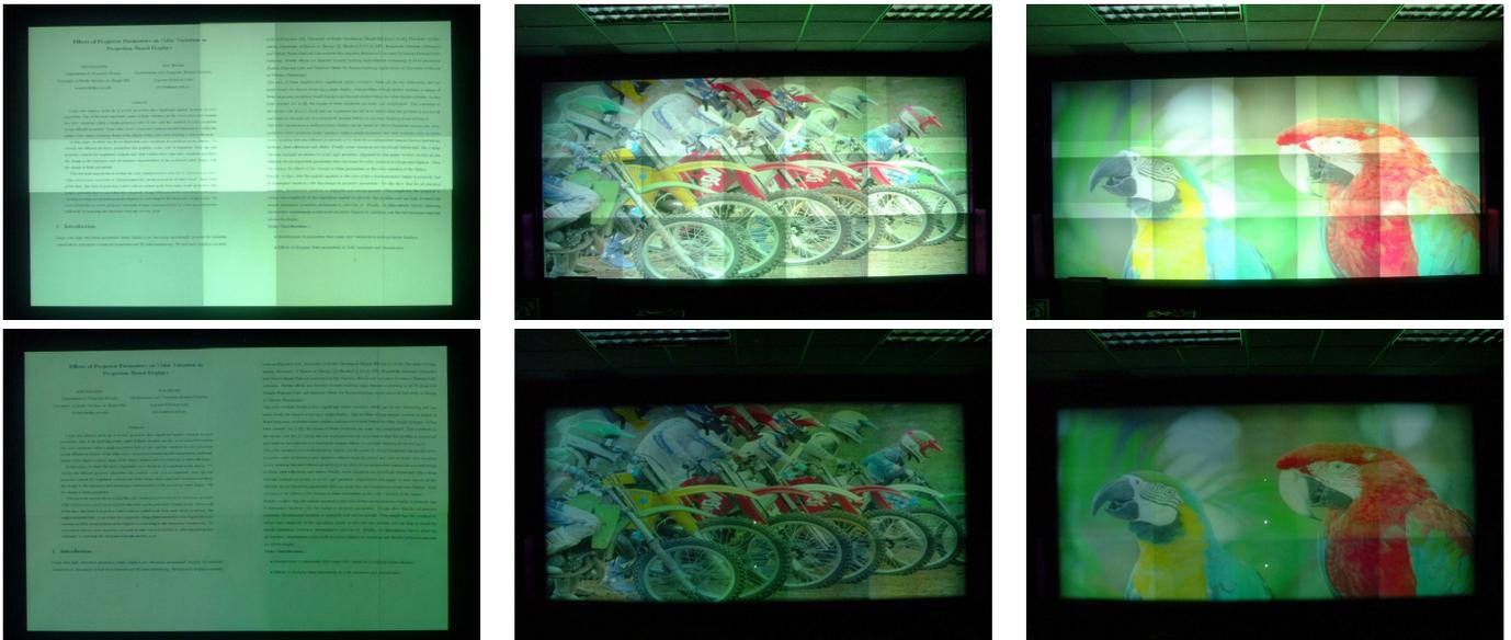
Fig. 16. The top row shows the image before correction, and the bottom row shows the image after luminance matching. Left column:  $2 \times 2$  array of four projectors. Right two columns:  $5 \times 3$  array of fifteen projectors
