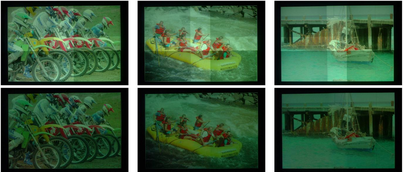
Fig. 15. The top row shows the image before correction, and the bottom row shows the image after luminance matching for  $2 \times 2$  array of four projectors.
