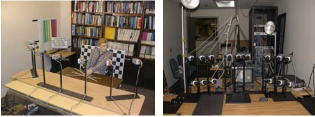
Figure 3: Camera acquisition arrays for 5 trinocular camera triples. (Left) Seven camera setup. (Right) 15 camera setup
