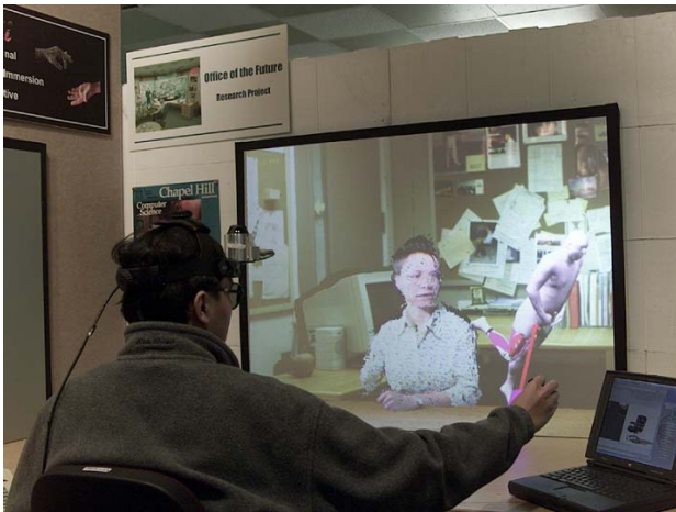
Figure 1: Our 3D tele-immersion realization with the local user manipulating the visible human data set using a virtual laser pointer. The local user sees the remote collaborator in perspective-correct 3D stereo, and both users are able to manipulate in 3D the shared visible human object.
