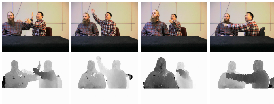
Figure 14: More results from our real-time online stereo system. The first row shows the input images; The second row shows the corresponding disparity map.
