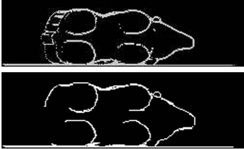
Figure 4: a) Registration points derived from curvature measures and b) space curve generated by linking curvature points.
