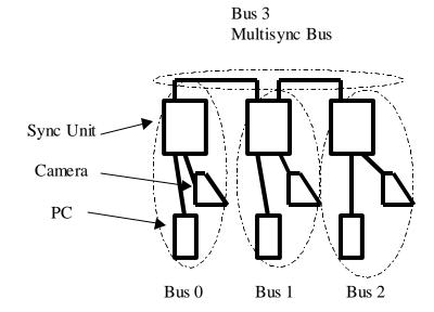
In order to use multiple sync units together (to increase the bandwidth), the sync units must be connected to each other to create an independent bus as shown in the diagram above. This bus will be the source for synchronizing the timing.
