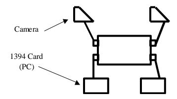
One connector will be connected to the Firewire card while the other can be connected to a camera or to another sync unit. It is important that the buses are not interconnected. For example, do not have one camera plugged into both buses at the same time.
