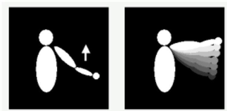
The most recent motion has the highest value, earlier motions have decreasing values subject to a threshold below which the value is set to zero. Different stages of creating and processing motion templates are described below.
