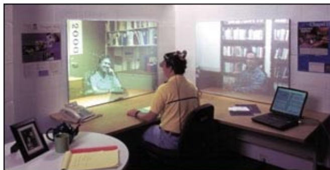
A University of North Carolina researcher meets virtually with colleagues from Pennsylvania and New York-life-size and in 3D. Tele-immersion's realtime rendering is accomplished through advanced computer vision, graphics, and network techniques.
