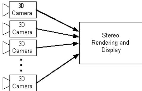
Figure 2: Tele-immersion framework with multiple view-independent streams mapped to the rendering-display node.
