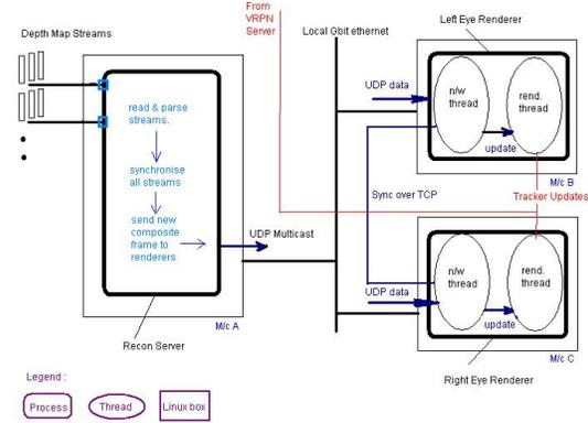
Figure 6: Tele-Immersion 3-PC Rendering Architecture.
