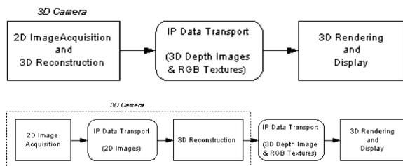
Figure 3: (a) 1-transport stage pipeline. (b) 2-transport stage pipeline where 3D camera functionality is split between two sites.
