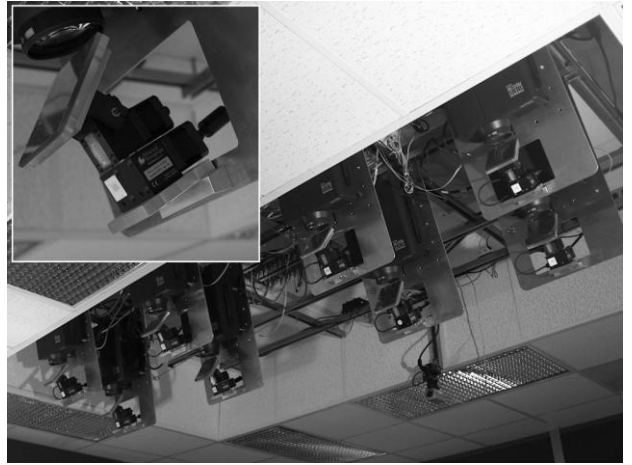
Figure 2: This image shows the PixelFlex projector array. The inset is a closeup view of the mirror and PTU in front of a projector.
