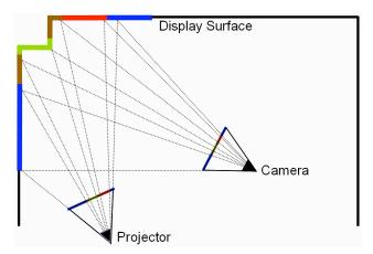
Figure 2. Mapping projector pixels to camera pixels.
